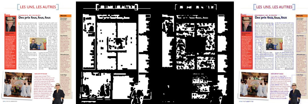
Figure 5. Document through different stages of processing: original, morphed Canny, morphed Canny with images removed and final output regions
